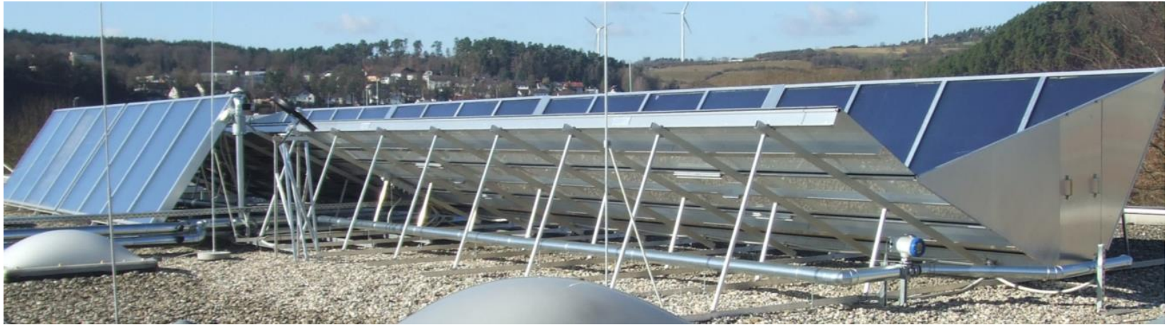
Reference flat-plates (glass-foil, front) and new RefleC-collectors (back)
